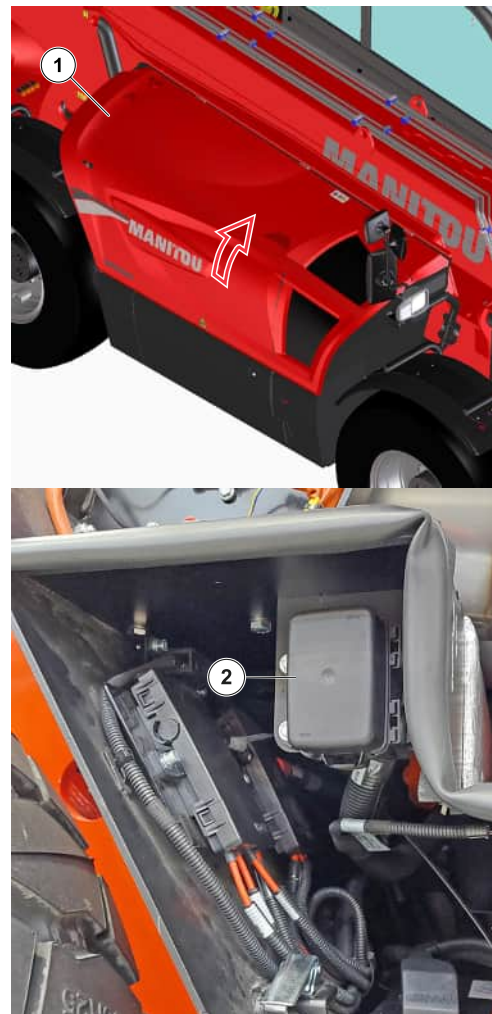
Figure 226: Fuse box and relays engine
