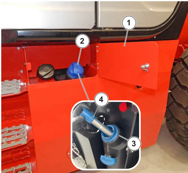
Figure 230: Checking and cleaning the DEF tank filler filter
