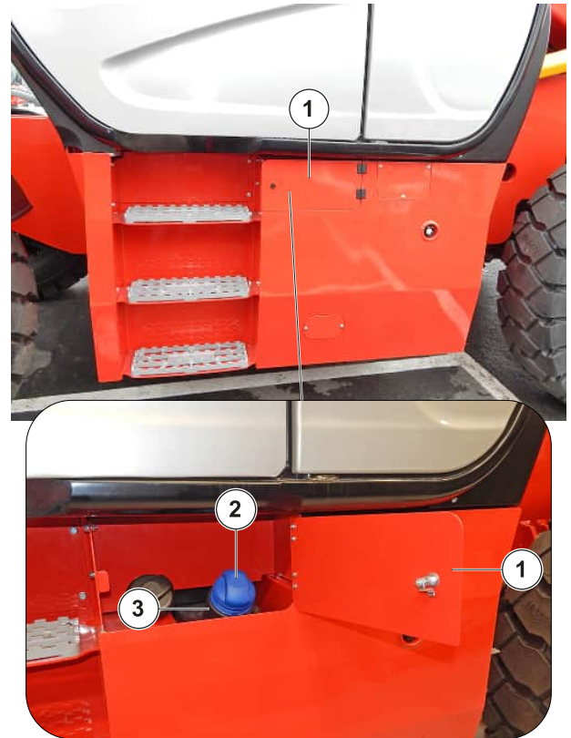
Figure 173: Checking DEF liquid level
