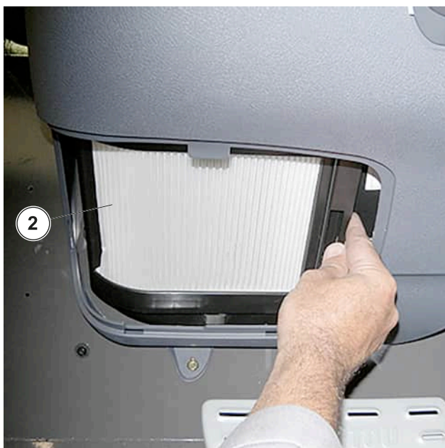
Figure 210: Ventilation filter inside the cabin
