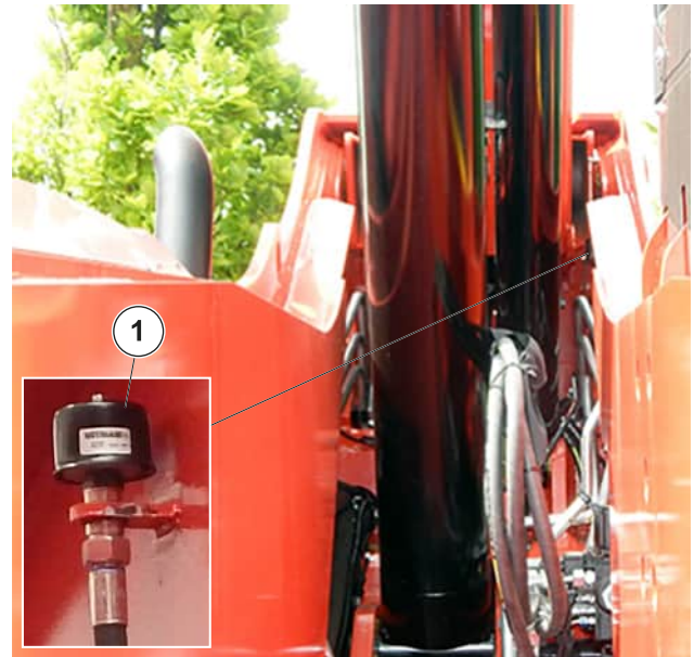
Figure 192: Replacing the hydraulic oil breather
