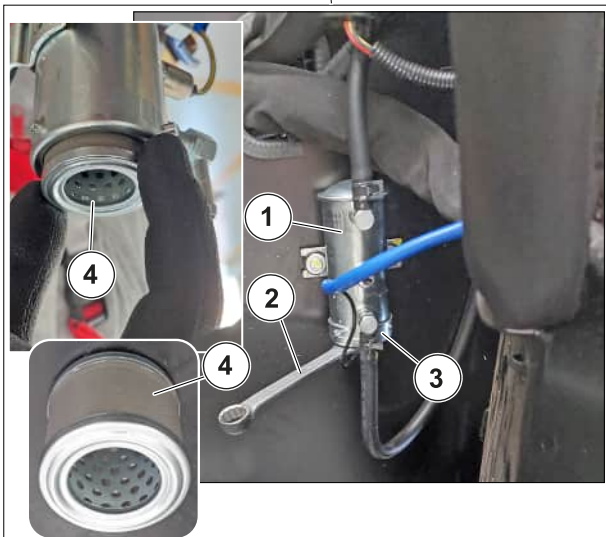
Figure 207: Fuel pump filter replacement
