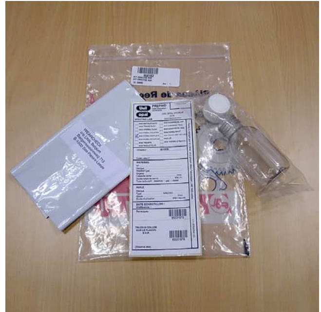
Figure 189: Hydraulic oil contamination check
