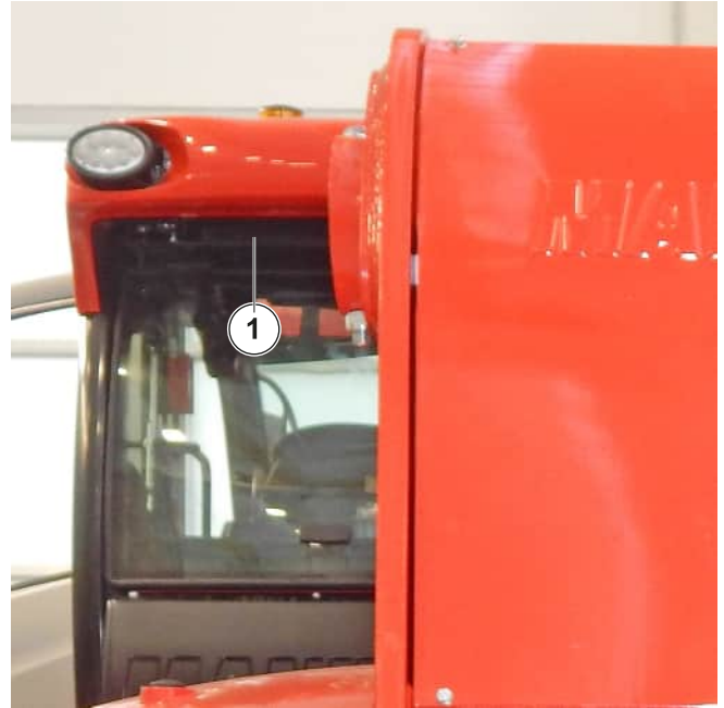
Figure 179: Air conditioning condenser grille
