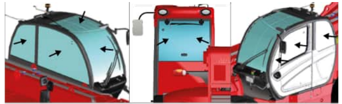
Figure 175: Cabin glass integrity check
